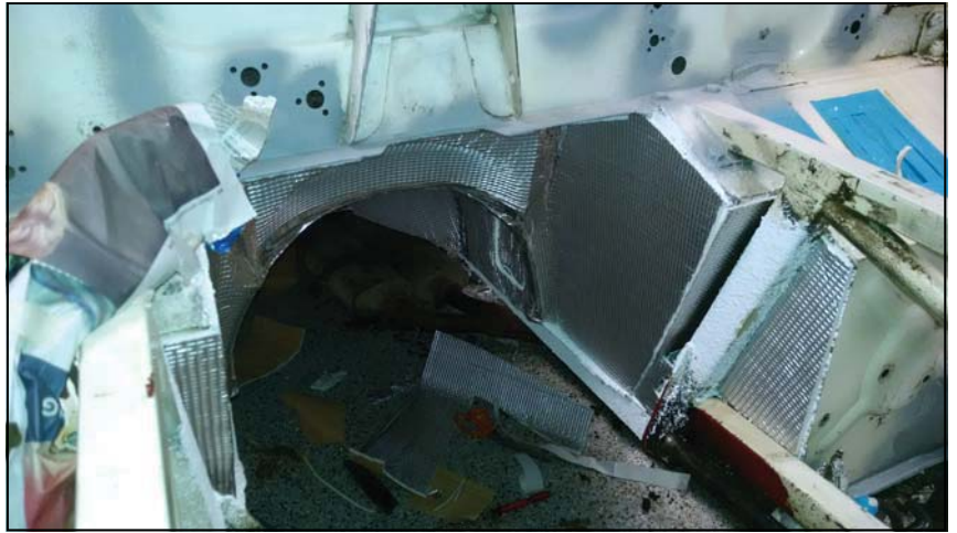
Transmission tunnel area insulated
