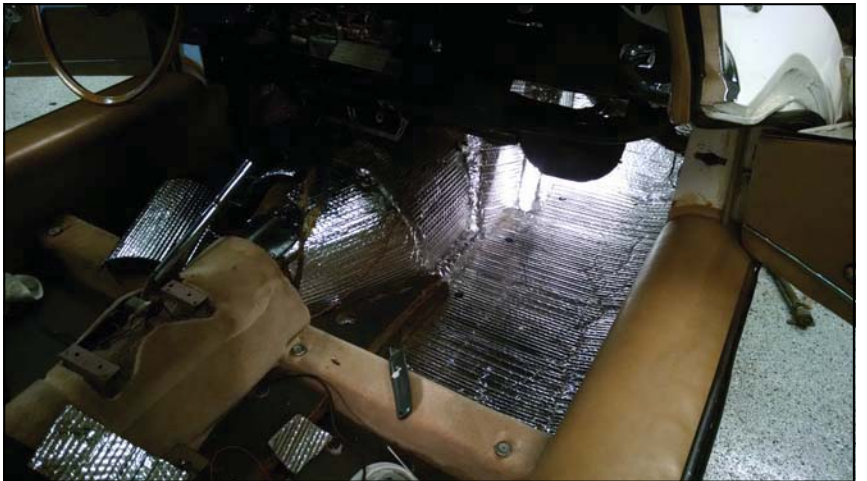
Interior area insulated with Reflectix.
